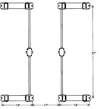
For installations in seismic active areas, optional earthquake safety straps are available. Order Model SS3600.
