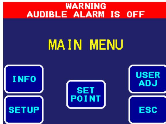
**Set Point:** This menu is password protected using the set point password (default 0000) accessible through the configuration menu. Danger and critical set-points are adjustable on a sensor by sensor basis. Up and down arrows navigate channel set-points. Pressing adj allows the up and down arrows to change the value then pressing enter(left arrow) saves the changes.
