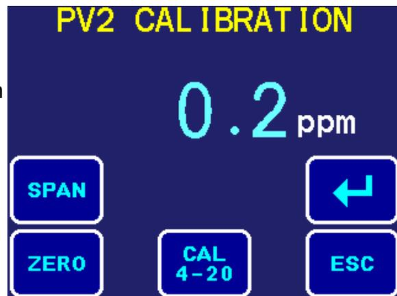
Process Output Calibration: This menu allows the 4 mA DC signal and 20 mA DC signal to be calibrated. It also allows a test of the outputs at 10 different select-able values from 4 mA to 20 mA.
