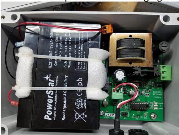
Note: The battery is shipped disconnected from the charging board
