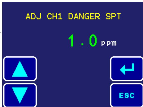
**Setup:** This menu is password protected (default 0000) and allows the calibration, configuration, and passwords to be set. Refer to the parameter list and calibration procedure sections of the manual for more information. The values in the calibration and configuration menus all follow the pattern of using the up and down arrows to navigate followed by pressing adjust to change them and then using the left arrow to save.
