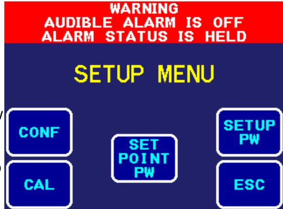
**Calibration(CAL):** This screen allows access to the calibration of both the sensor inputs (PVx/CHx) and the 4-20 mA DC outputs (POx) of the instruments.
