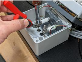
Loosen the setscrew holding the load cell. Remove the cell.
