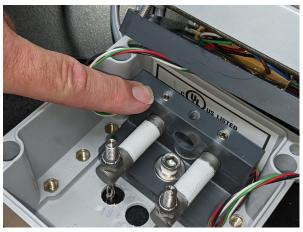
Check the new load cell. It should have "TOP" or a "T" written on it to show which side faces up when installed. If not, install it so the serial number on the side is right side up. Reverse these steps to install the new load cell.
