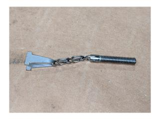
Use pliers to hold the bolt under the load cell and remove the nut. Don't let the bolt fall through the
