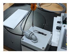
Disconnect the load cell that needs to be replaced from the terminal block. Loosen the strain relief on
